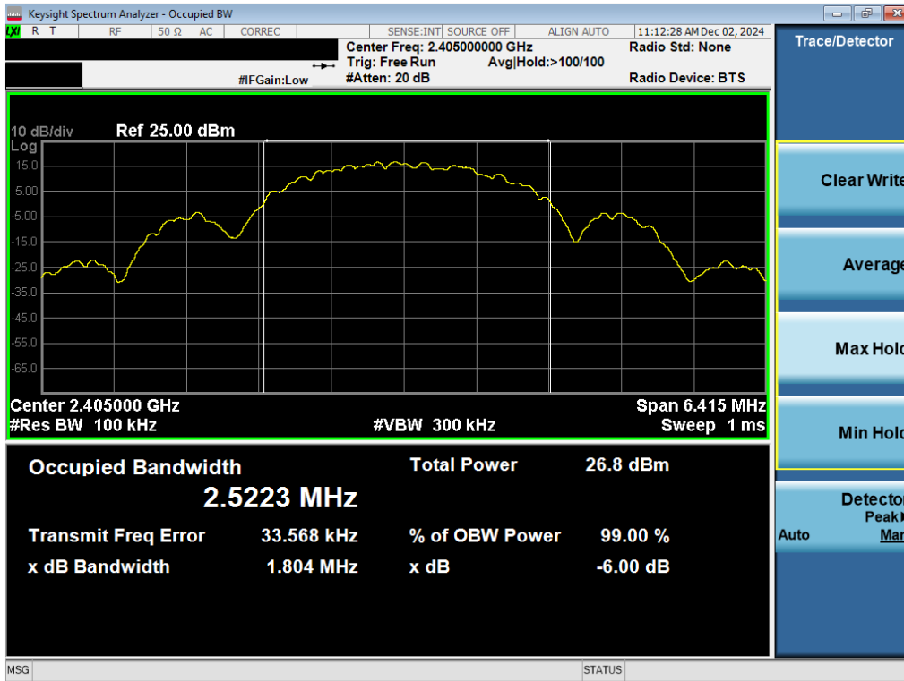
Plot 7-1. 6dB BW & 99% OBW Antenna WF7b (802.15.4, Ch. 11)
