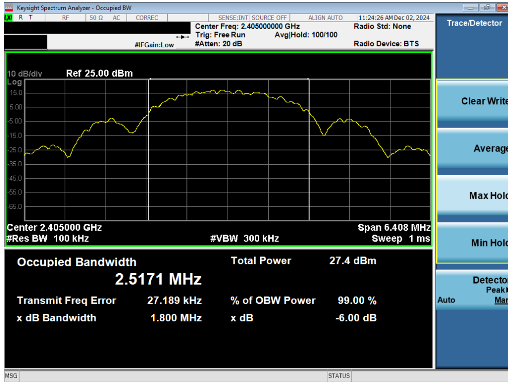
Plot 7-4. 6dB BW & 99% OBW Antenna WF2b (802.15.4, Ch. 11)
