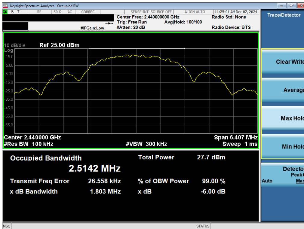
Plot 7-5. 6dB BW & 99% OBW Antenna WF2b (802.15.4, Ch. 18)
