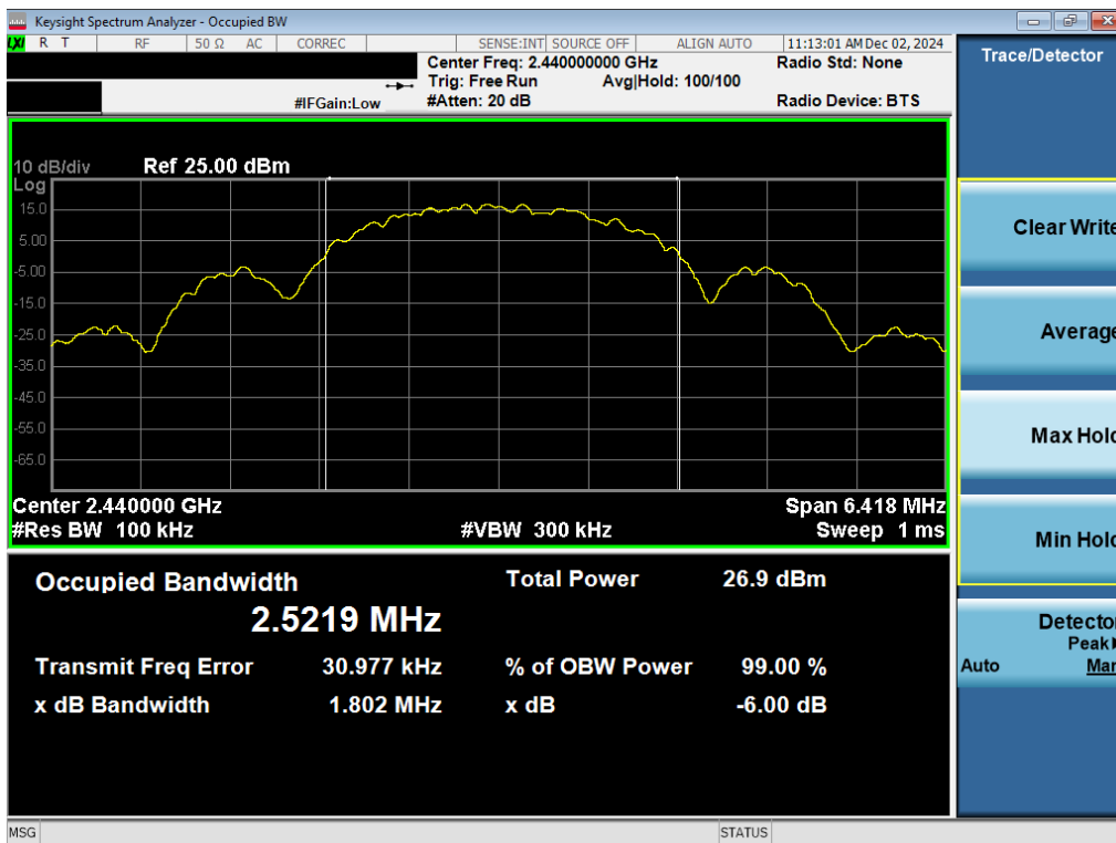
Plot 7-2. 6dB BW & 99% OBW Antenna WF7b (802.15.4, Ch. 18)
