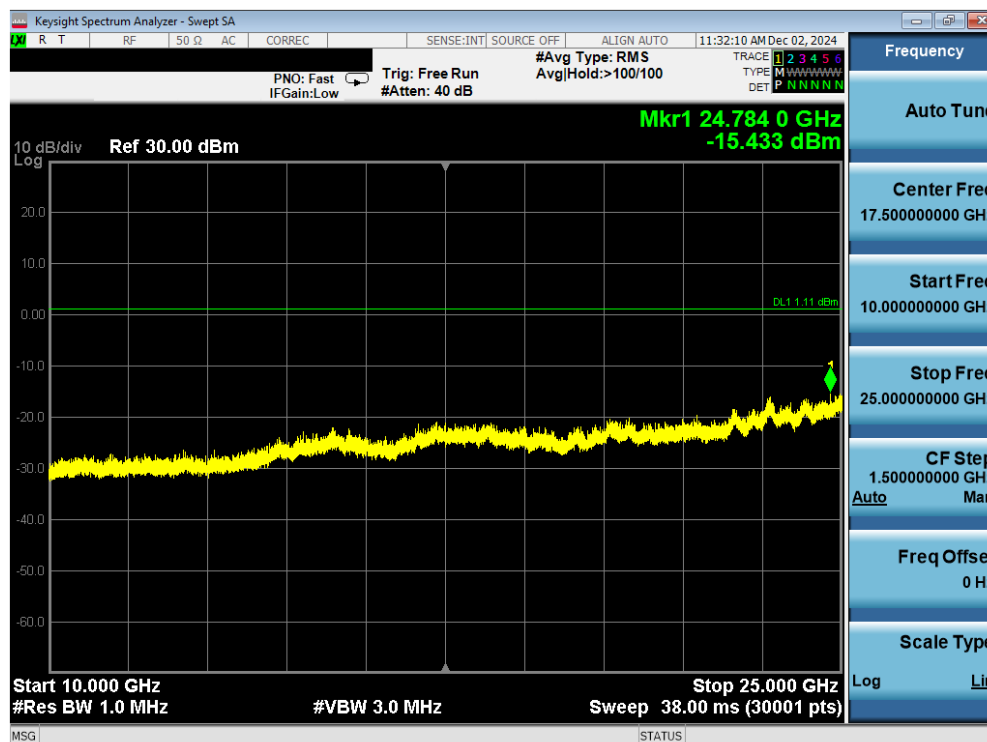
Plot 7-30. Conducted Spurious Antenna WF2b (802.15.4, ePA – Ch. 11)
