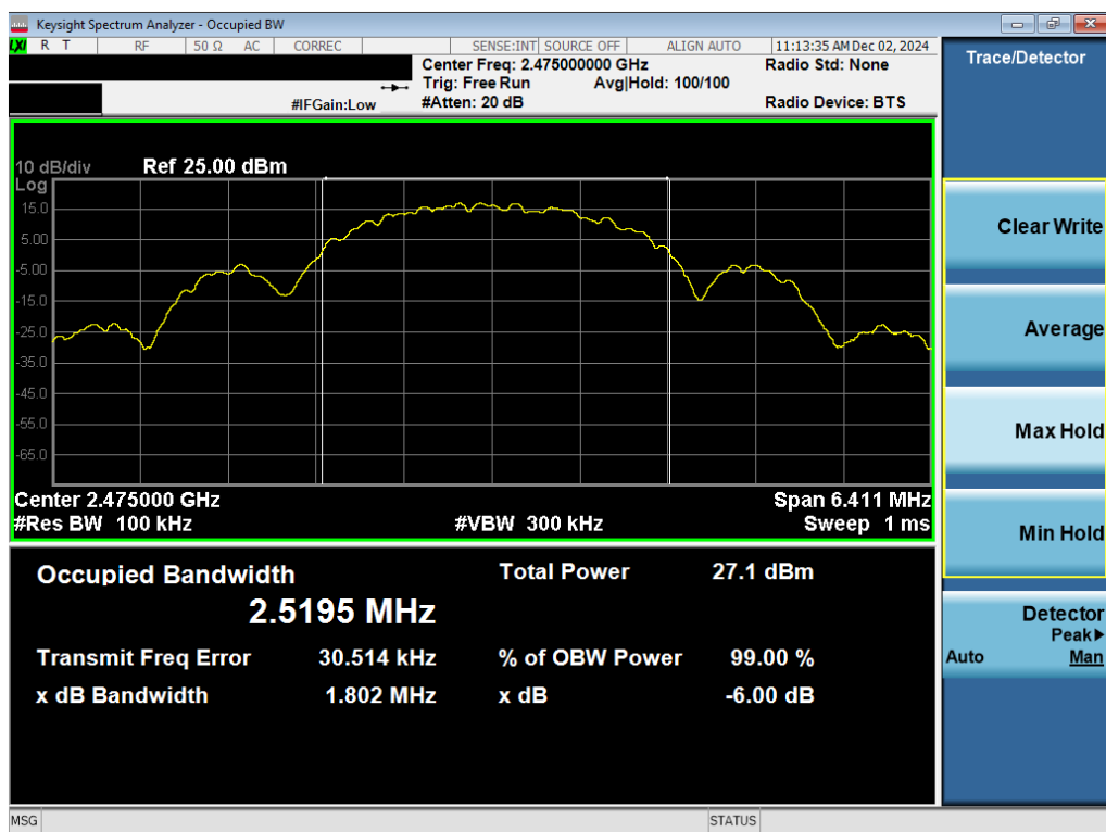
Plot 7-3. 6dB BW & 99% OBW Antenna WF7b (802.15.4, Ch. 25)
