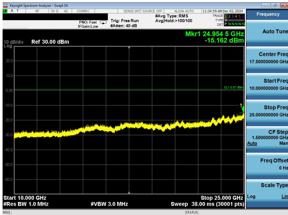
Plot 7-34. Conducted Spurious Antenna WF2b (802.15.4, ePA – Ch. 25)
