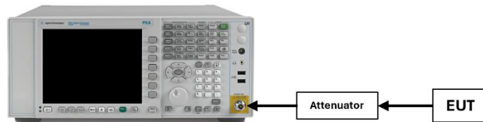
Figure 7-5. Test Instrument & Measurement Setup
