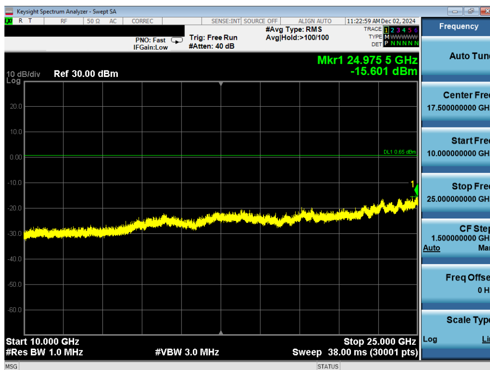
Plot 7-28. Conducted Spurious Antenna WF7b (802.15.4, ePA – Ch. 25)
