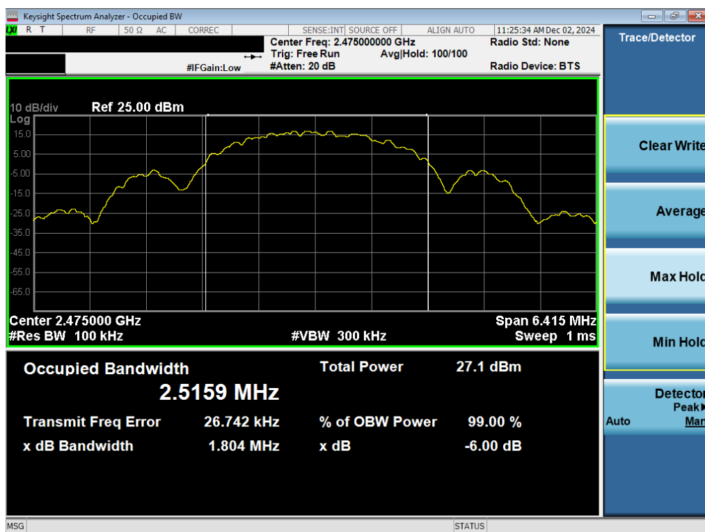
Plot 7-6. 6dB BW & 99% OBW Antenna WF2b (802.15.4, Ch. 25)
