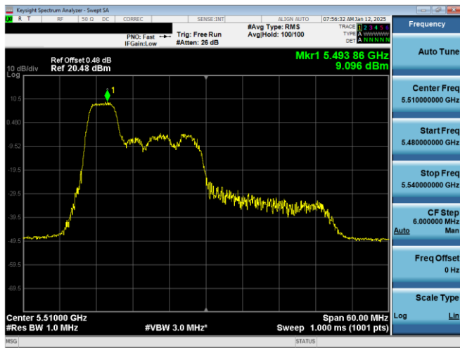
Plot 7-19. PSD Antenna WF2a (40MHz BW 11ax Index37 – RU52 – Ch.102)
