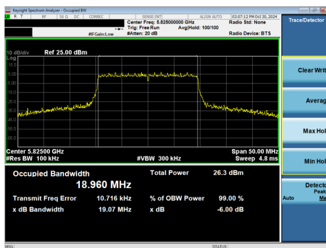
Plot 7-12. 6dB BW & 99% OBW Antenna WF7b (20MHz BW 11ax– RU242 – Ch.165)
