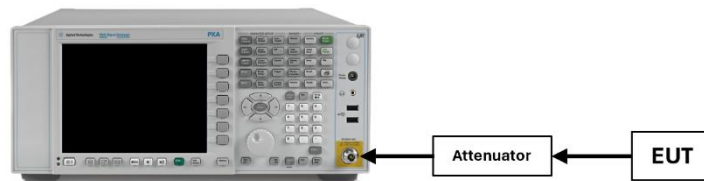
Figure 7-1. Test Instrument & Measurement Setup
