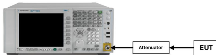
Figure 7-2. Test Instrument & Measurement Setup
