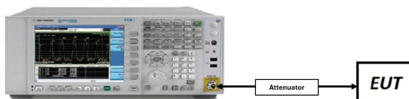
Figure 7-1. Test Instrument & Measurement Setup
