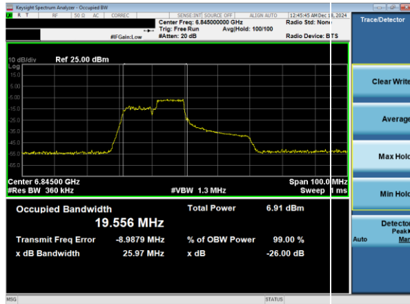
Plot 7-26. 26dB & 99% Bandwidth Plot Antenna WF7a (40MHz 802.11ax RU106 (UNII Band 7) – Ch. 179)
