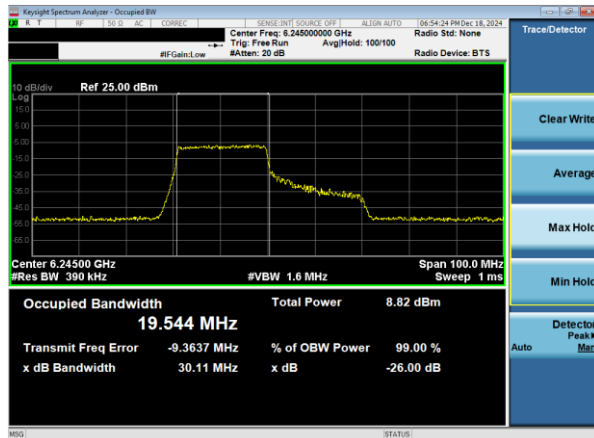
Plot 7-2. 26dB & 99% Bandwidth Plot Antenna WF8 (40MHz 802.11ax RU242 (UNII Band 5) – Ch. 59)
