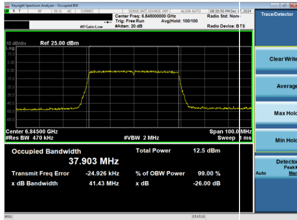
Plot 7-14. 26dB & 99% Bandwidth Plot Antenna WF8 (40MHz 802.11ax RU484 (UNII Band 7) – Ch. 179)
