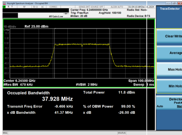
Plot 7-22. 26dB & 99% Bandwidth Plot Antenna WF7a (40MHz 802.11ax RU484 (UNII Band 5) – Ch. 59)
