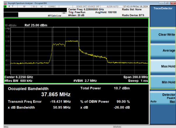
Plot 7-19. 26dB & 99% Bandwidth Plot Antenna WF7a (80MHz 802.11ax RU242 (UNII Band 5) – Ch. 55)
