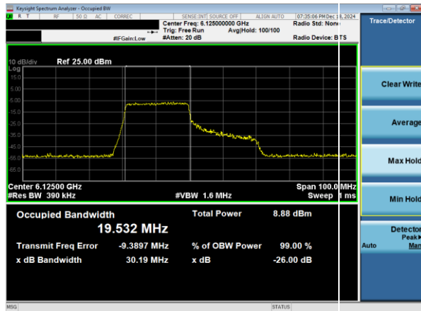
Plot 7-18. 26dB & 99% Bandwidth Plot Antenna WF7a (40MHz 802.11ax RU242 (UNII Band 5) – Ch. 35)
