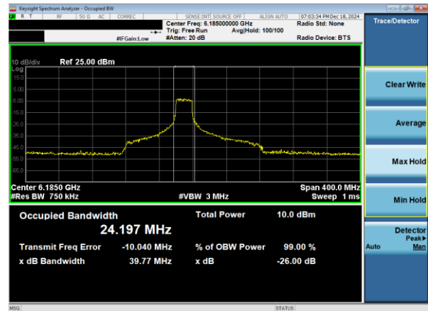
Plot 7-4. 26dB & 99% Bandwidth Plot Antenna WF8 (160MHz 802.11ax RU242 (UNII Band 5) – Ch. 47)
