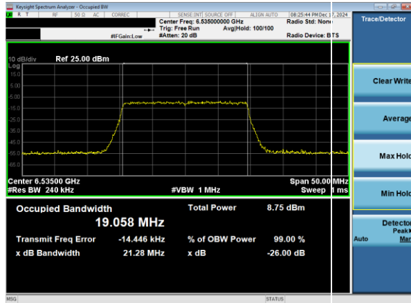
Plot 7-13. 26dB & 99% Bandwidth Plot Antenna WF8 (20MHz 802.11ax RU242 (UNII Band 7) – Ch. 117)
