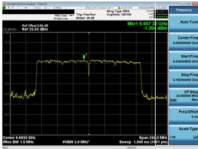
Plot 7-271. PSD Plot CDD Antenna WF8 (160MHz 802.11ax RU996x2 (UNII Band 7) – Ch. 143)
