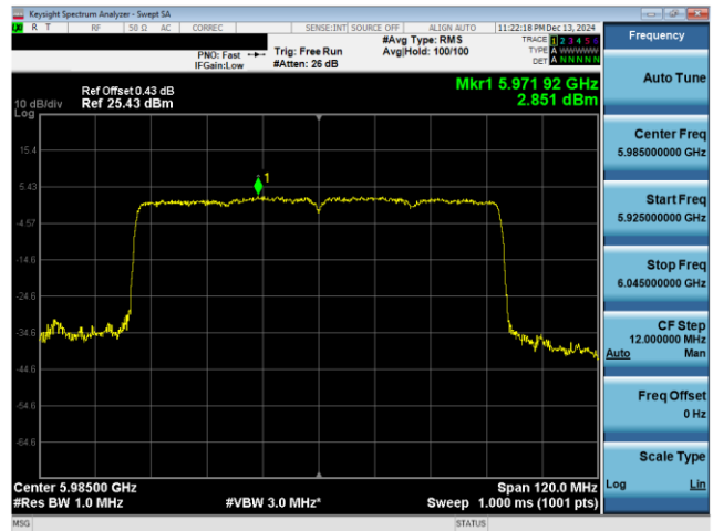
Plot 7-238. PSD Plot CDD Antenna WF7a (80MHz 802.11ax RU996 (UNII Band 5) – Ch. 7)
