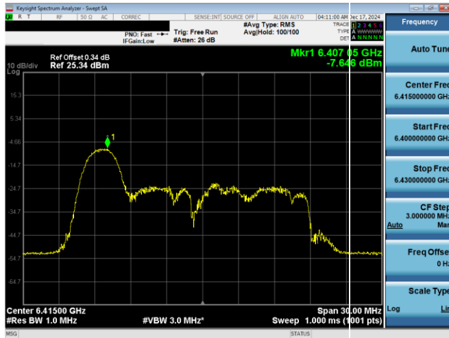
Plot 7-193. PSD Plot Antenna WF7a (20MHz 802.11ax RU26 (UNII Band 5) – Ch. 93)
