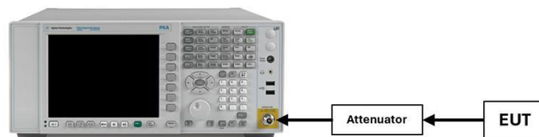
Figure 7-1. Test Instrument & Measurement Setup
