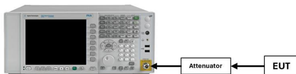
Figure 7-2. Test Instrument & Measurement Setup
