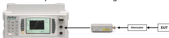
Figure 7-3. Test Instrument & Measurement Setup
