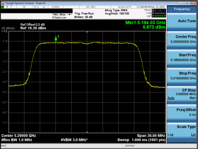
Plot 7-20. PSD Antenna WF7a (20MHz BW 11ax– RU242 – Ch.40)
