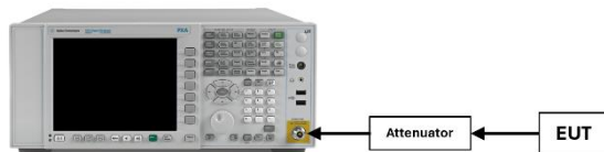
Figure 7-4. Test Instrument & Measurement Setup
