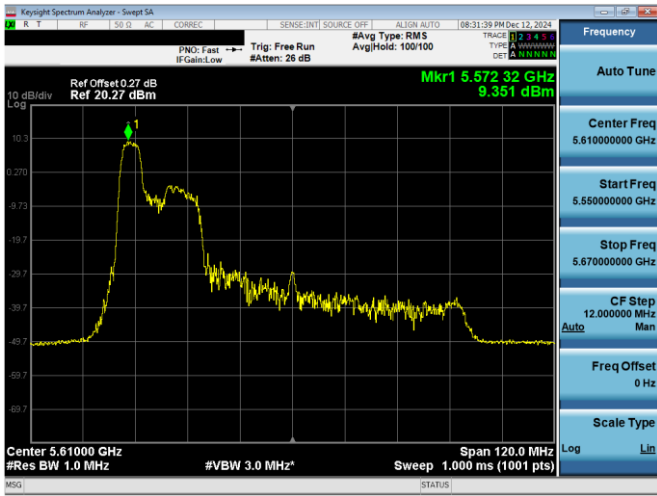
Plot 7-15. PSD Antenna WF7a (80MHz BW 11ax Index37 – RU52 – Ch.122)
