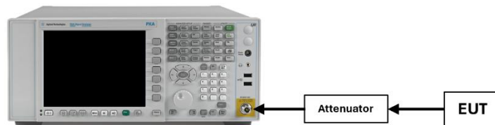
Figure 7-1. Test Instrument & Measurement Setup
