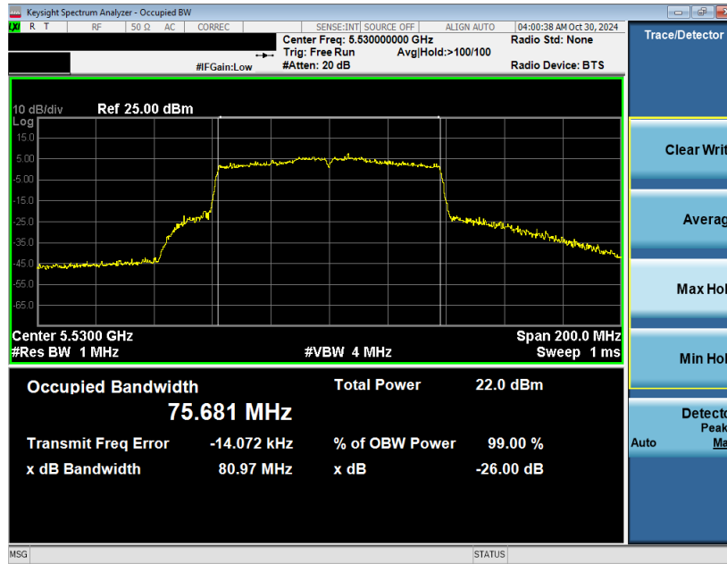
Plot 7-3. 26dB BW & 99% OBW Antenna WF8 (80MHz BW 802.11ac – Ch. 106)
