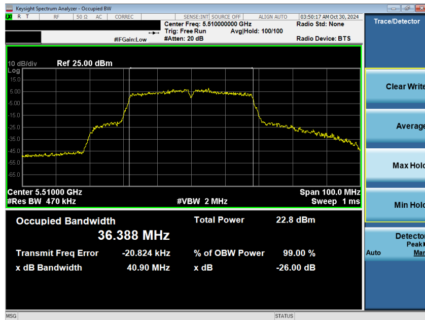
Plot 7-2. 26dB BW & 99% OBW Antenna WF8 (40MHz BW 802.11n – Ch. 102)
