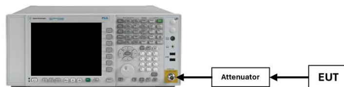
Figure 7-5. Test Instrument & Measurement Setup
