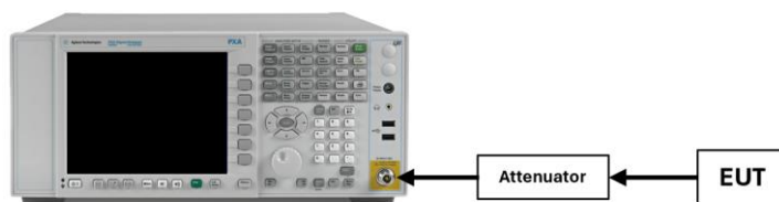
Figure 7-3. Test Instrument & Measurement Setup
