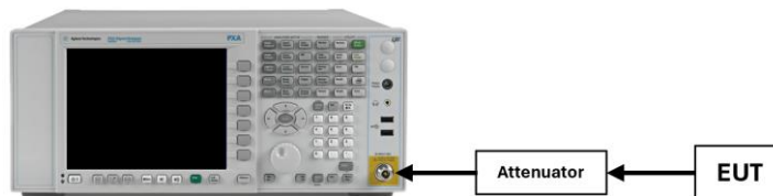
Figure 7-6. Test Instrument & Measurement Setup
