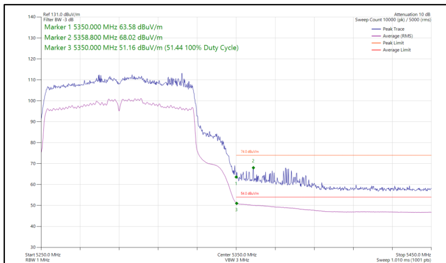
Figure 190 - 802.11ac VHT80, TxBF, Core 0 - Core 1 - 5290 MHz Band Edge Frequency 5350 MHz
