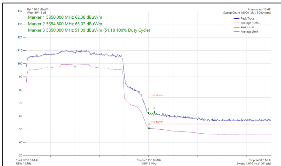
Figure 157 - 802.11ax HE80, SU, SISO, Core 0 - 5290 MHz Band Edge Frequency 5350 MHz
