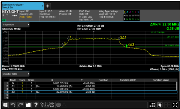
Figure 312 - 802.11n HT20 Maximum 26 dB EBW
