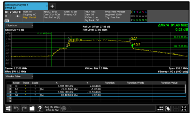
Figure 341 - 802.11ac VHT80 Maximum 99% OBW
