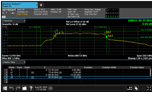
Figure 340 - 802.11ac VHT80 Minimum 99% OBW
