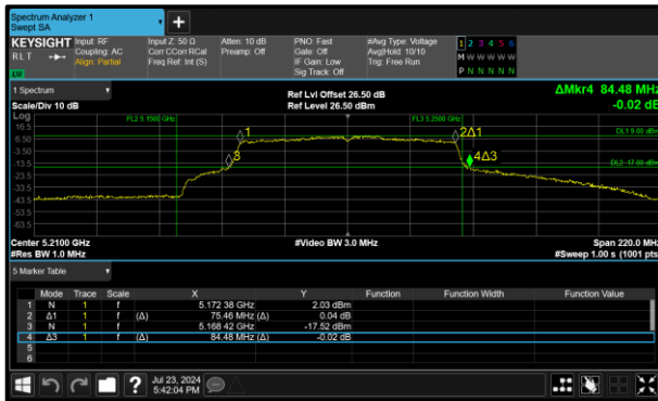
Figure 324 - 802.11ac VHT80 Minimum 99% OBW
