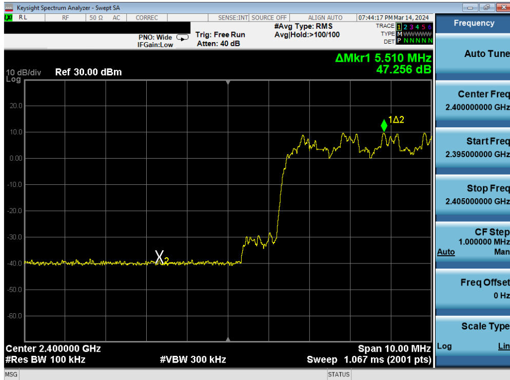
Plot 7-13. Band Edge Plot (Bluetooth with Hopping Enabled, 8DPSK,)
