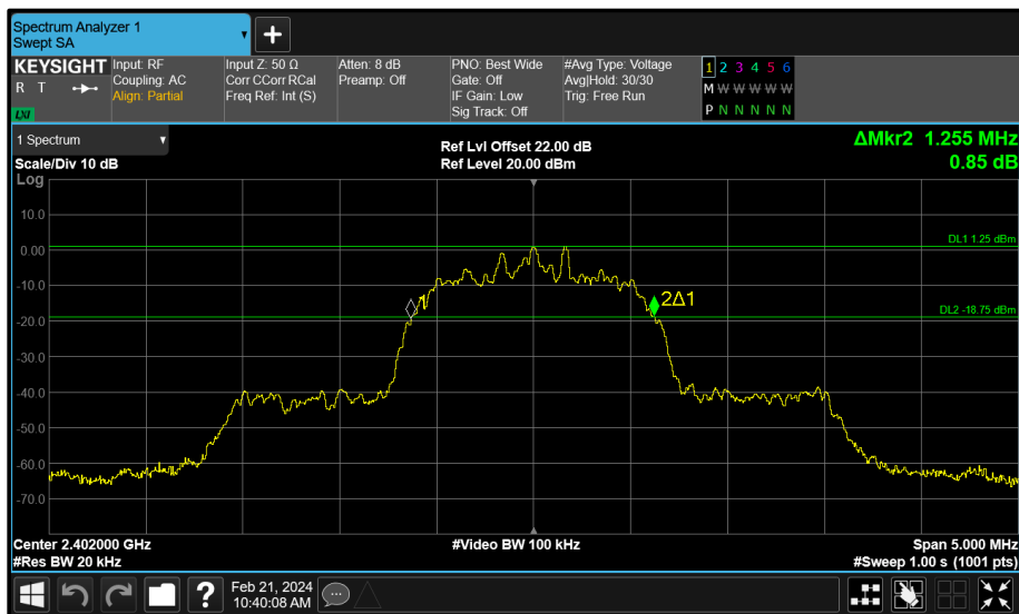
Figure 22 - Core 0 (A) 2402 MHz (CH0) 20 dB Bandwidth
