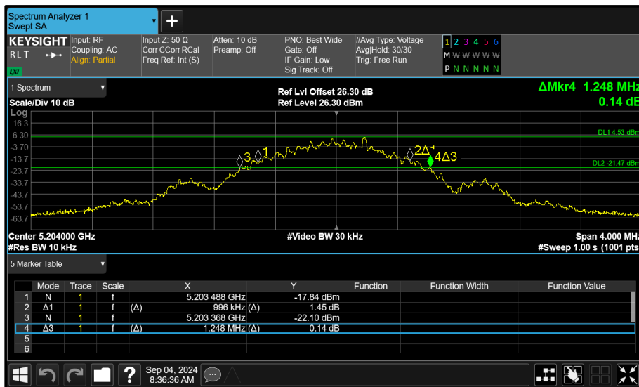
Figure 32 - Core 0 (A) 5204 MHz (CH54) 26 dB and 99% Bandwidth
