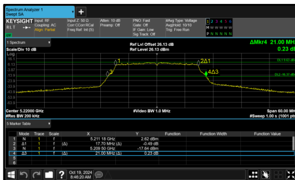
Figure 276 - 802.11n HT20 Minimum 99% OBW
