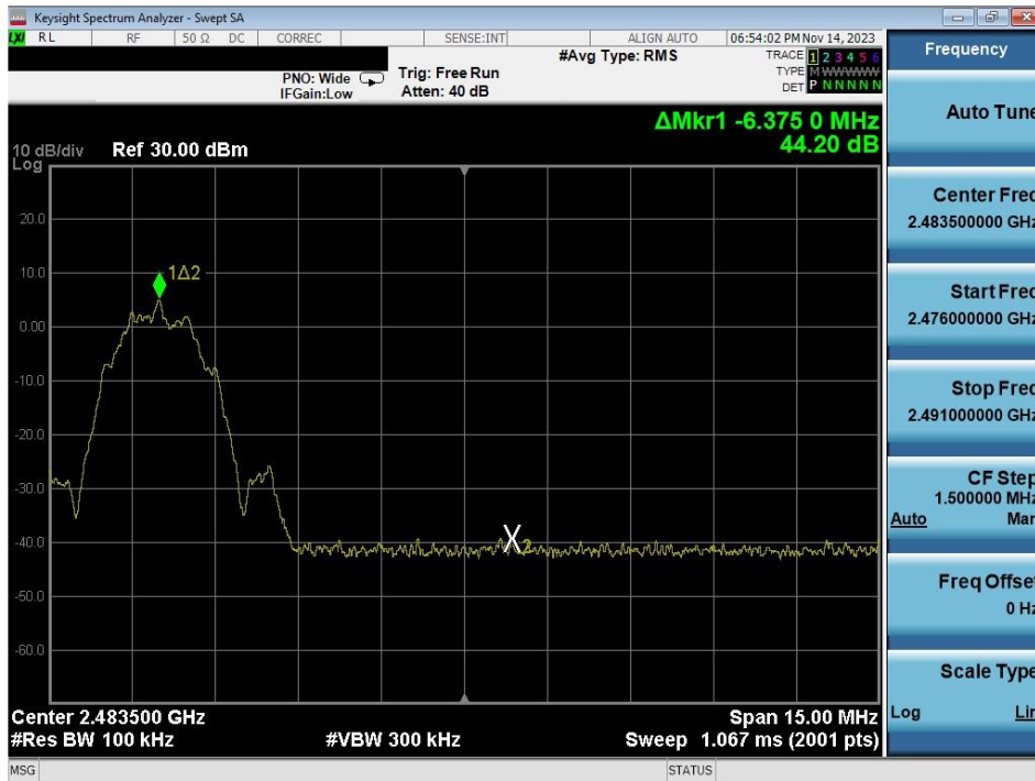
Plot 7-16. Band Edge Plot (Bluetooth (LE), 2Mbps – Ch. 38)
