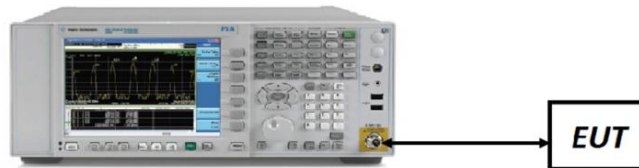
Figure 7-4. Test Instrument & Measurement Setup
