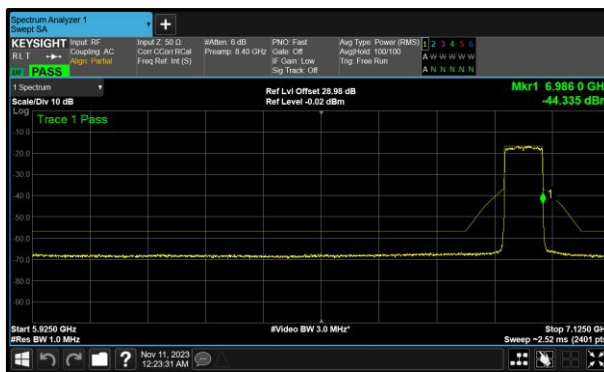
Figure 205 - A(Core 0) 802.11ax HE80 SU LPI 6945 MHz (CH199)
