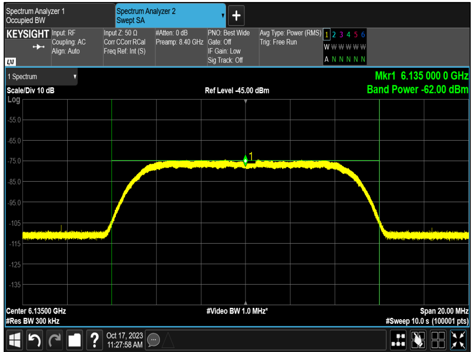
Figure 193 - Example of AWGN Signal
