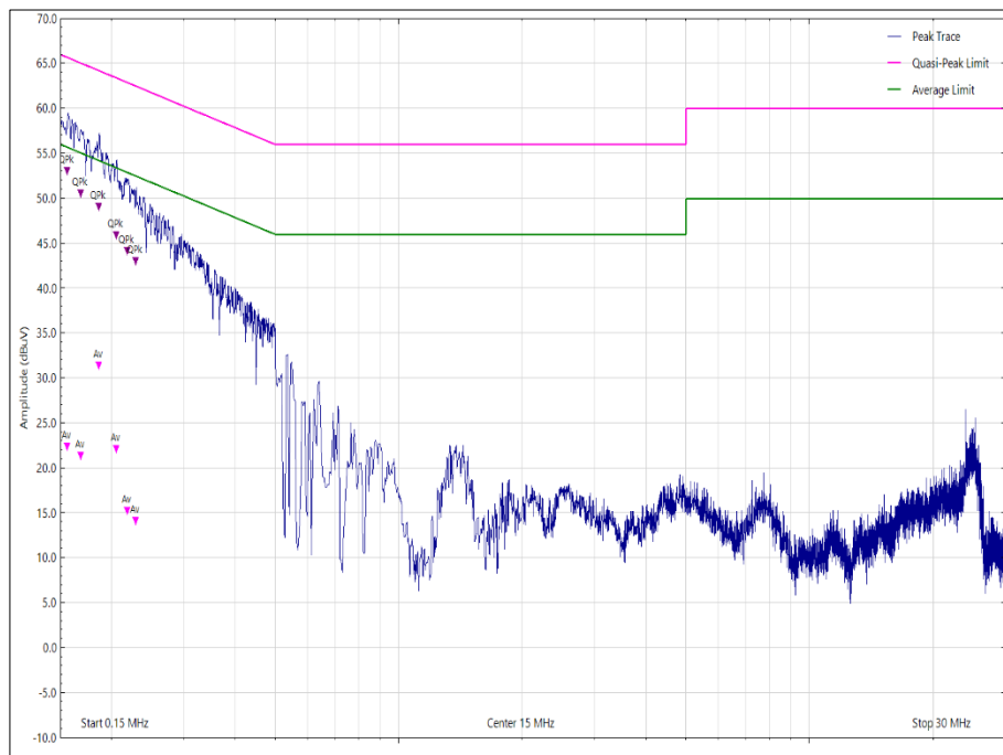
Figure 5 - Neutral Line - 150 kHz to 30 MHz
