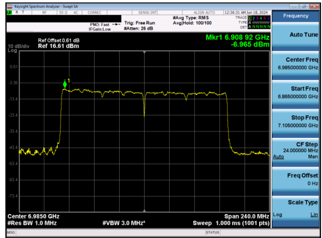
Plot 7-954. LPI Power Spectral Density Plot SDM Antenna 1b (160MHz 802.11ax RU996x2 (UNII Band 8) – Ch. 207)
