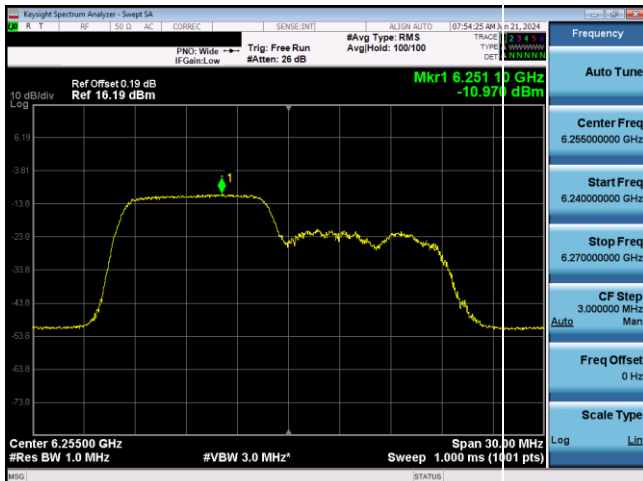
Plot 7-985. VLP Power Spectral Density Plot Antenna 3b (20MHz 802.11ax RU106 (UNII Band 5) – Ch. 61)
