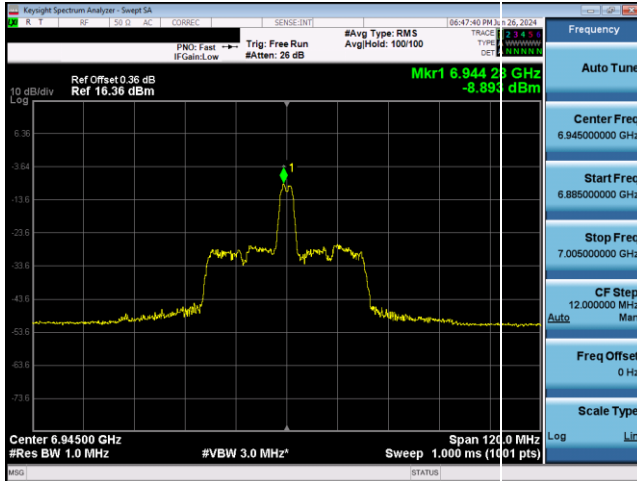
Plot 7-877. LPI Power Spectral Density Plot SDM Antenna 5T (80MHz 802.11ax RU26 (UNII Band 8) – Ch. 199)
