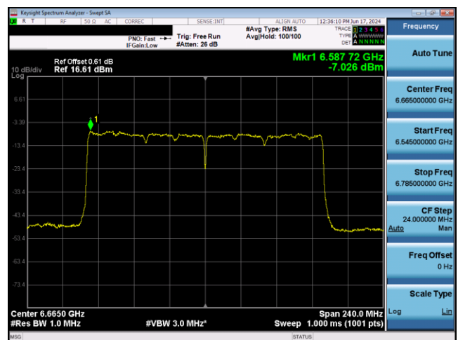
Plot 7-858. LPI Power Spectral Density Plot SDM Antenna 3b (160MHz 802.11ax RU996x2 (UNII Band 7) – Ch. 143)
