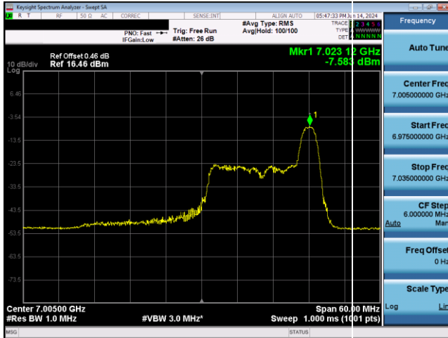
Plot 7-871. LPI Power Spectral Density Plot SDM Antenna 5T (40MHz 802.11ax RU26 (UNII Band 8) – Ch. 211)
