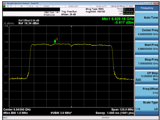
Plot 7-758. LPI Power Spectral Density Plot Antenna 1b (80MHz 802.11ax RU996 (UNII Band 8) – Ch. 199)
