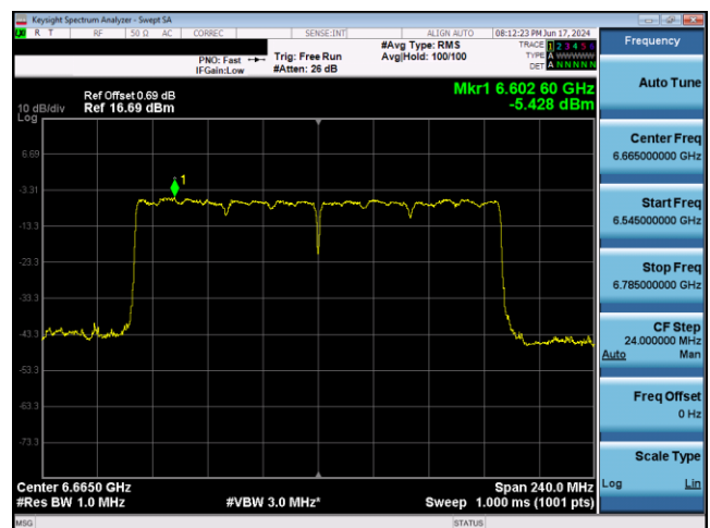
Plot 7-746. LPI Power Spectral Density Plot Antenna 1b (160MHz 802.11ax RU996x2 (UNII Band 7) – Ch. 143)
