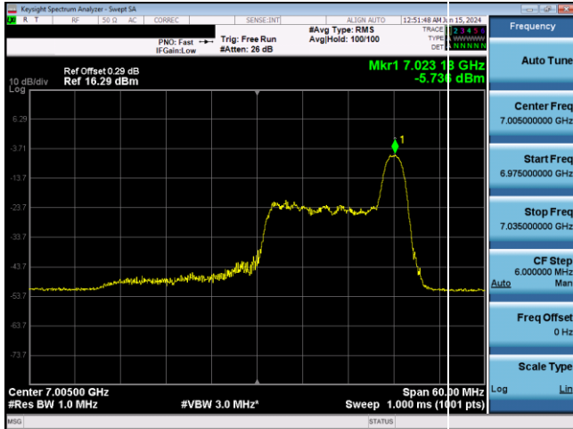
Plot 7-689. LPI Power Spectral Density Plot Antenna 3b (40MHz 802.11ax RU26 (UNII Band 8) - Ch. 211)
