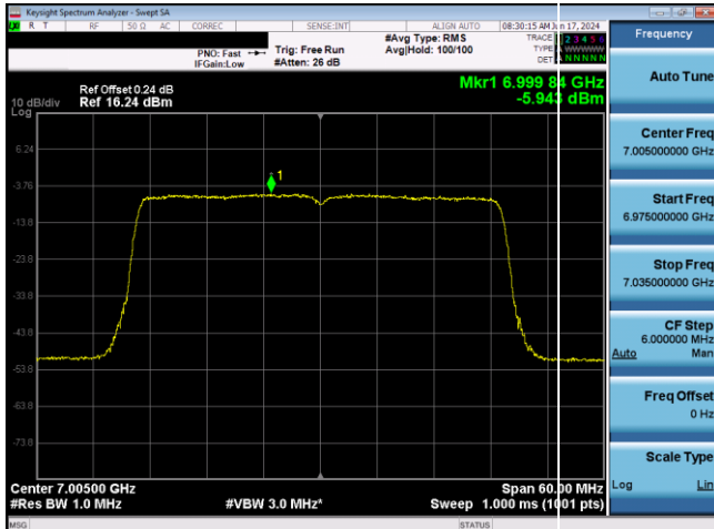
Plot 7-690. LPI Power Spectral Density Plot Antenna 3b (40MHz 802.11ax RU484 (UNII Band 8) - Ch. 211)
