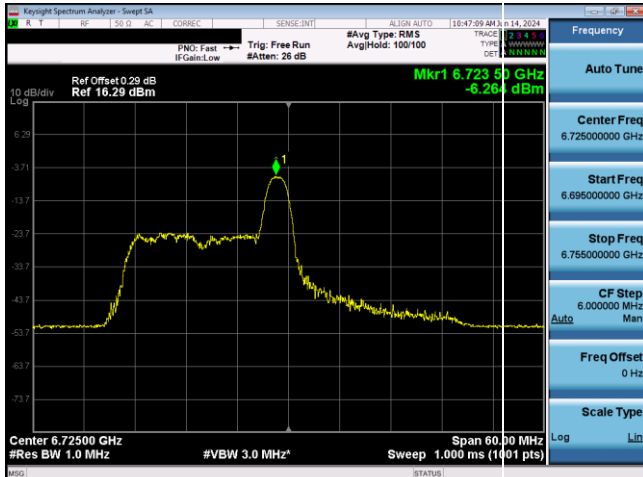
Plot 7-608. LPI Power Spectral Density Plot Antenna 5T (40MHz 802.11ax RU26 (UNII Band 7) – Ch. 155)
