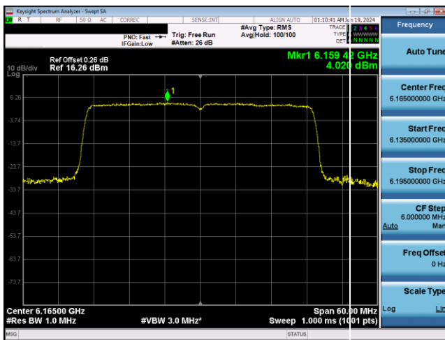
Plot 7-546. SP Power Spectral Density Plot CDD Antenna 1b (40MHz 802.11ax RU484 (UNII Band 5) - Ch. 43)
