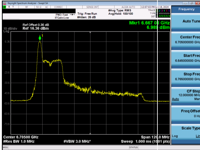
Plot 7-523. SP Power Spectral Density Plot CDD Antenna 5T (80MHz) 802.11ax RU26 (UNII Band 7) – Ch. 151
