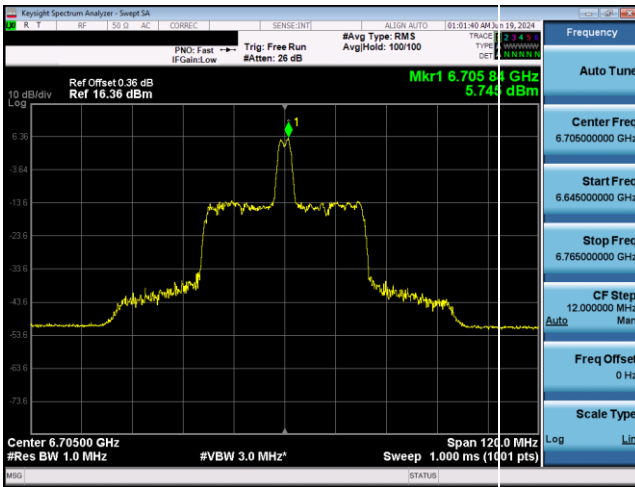
Plot 7-564. SP Power Spectral Density Plot CDD Antenna 1b (80MHz 802.11ax RU26 (UNII Band 7) - Ch. 151)
