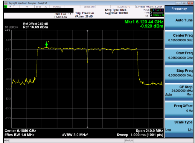
Plot 7-426. SP Power Spectral Density Plot Antenna 3b (160MHz 802.11ax RU996x2 (UNII Band 5) – Ch. 47)
