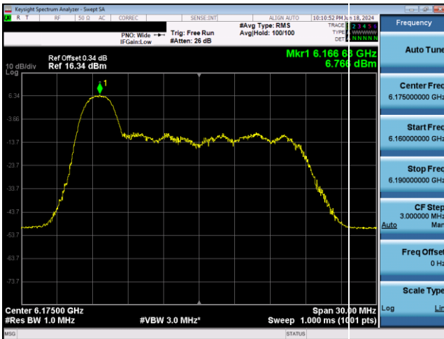
Plot 7-443. SP Power Spectral Density Plot Antenna 1b (20MHz 802.11ax RU26 (UNII Band 5) – Ch. 45)
