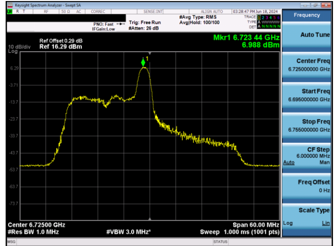
Plot 7-432. SP Power Spectral Density Plot Antenna 3b (40MHz 802.11ax RU26 (UNII Band 7) – Ch. 155)
