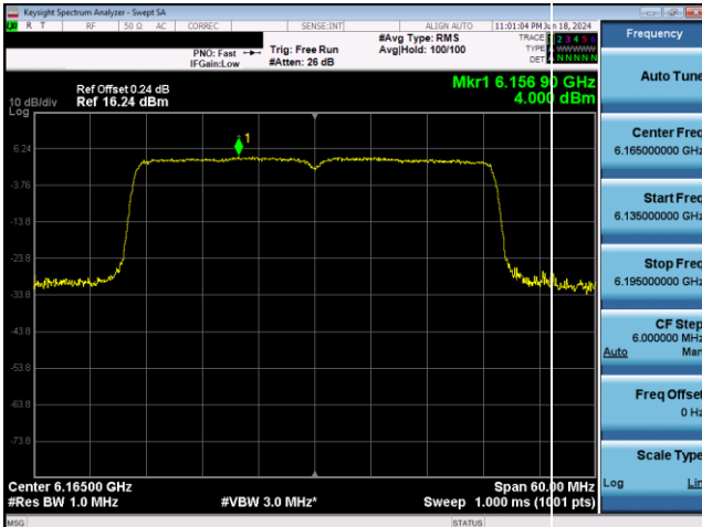
Plot 7-450. SP Power Spectral Density Plot Antenna 1b (40MHz 802.11ax RU484 (UNII Band 5) – Ch. 43)
