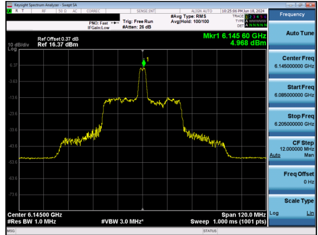
Plot 7-452. SP Power Spectral Density Plot Antenna 1b (80MHz 802.11ax RU26 (UNII Band 5) – Ch. 39)
