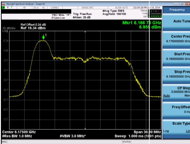
Plot 7-411. SP Power Spectral Density Plot Antenna 3b (20MHz 802.11ax RU26 (UNII Band 5) – Ch. 45)
