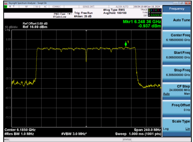
Plot 7-394. SP Power Spectral Density Plot Antenna 5T (160MHz 802.11ax RU996x2 (UNII Band 5) – Ch. 47)
