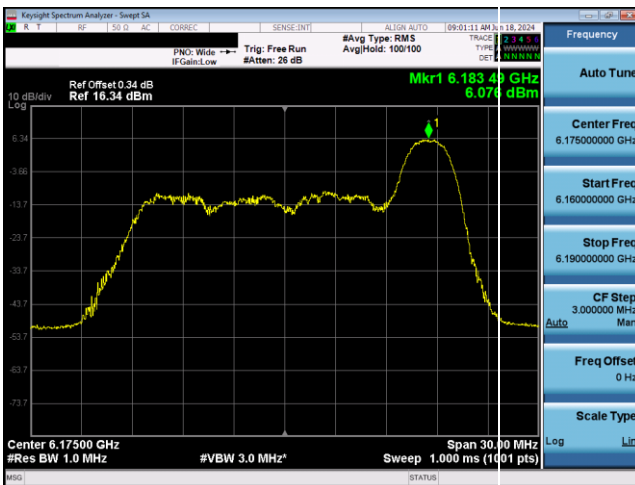
Plot 7-381. SP Power Spectral Density Plot Antenna 5T (20MHz 802.11ax RU26 (UNII Band 5) – Ch. 45)
