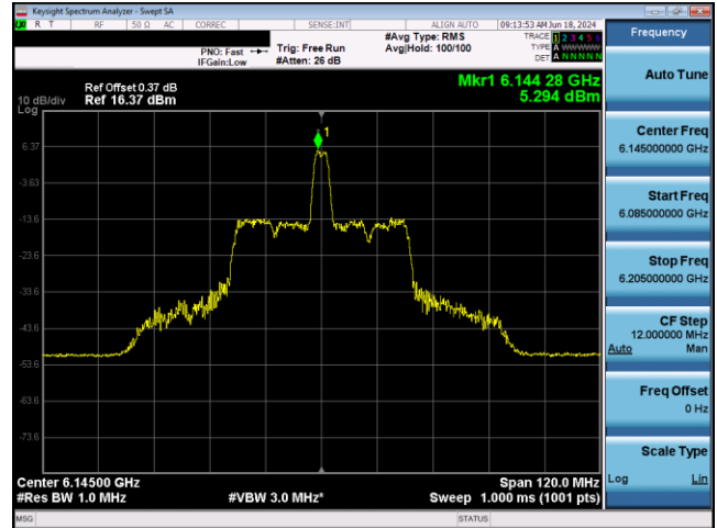
Plot 7-388. SP Power Spectral Density Plot Antenna 5T (80MHz 802.11ax RU26 (UNII Band 5) – Ch. 39)
