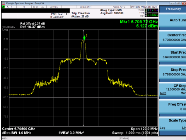
Plot 7-404. SP Power Spectral Density Plot Antenna 5T (80MHz 802.11ax RU26 (UNII Band 7) - Ch. 151)
