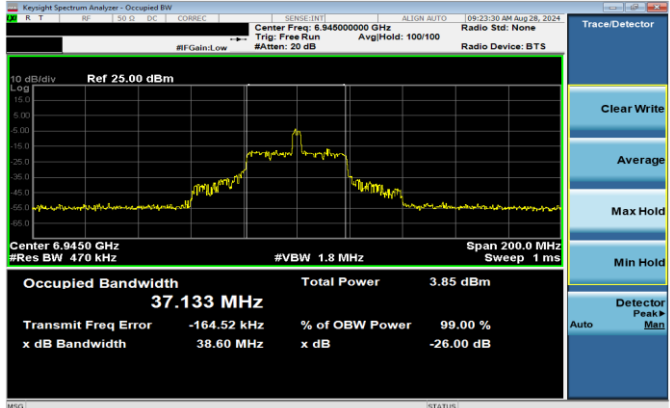
Plot 7-282. 26dB & 99% Bandwidth Plot Antenna 1b LPI (80MHz 802.11ax RU26 (UNII Band 8) – Ch. 199)
