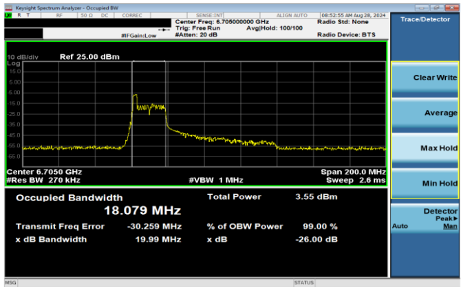
Plot 7-265. 26dB & 99% Bandwidth Plot Antenna 1b LPI (80MHz 802.11ax RU26 (UNII Band 7) – Ch. 151)
