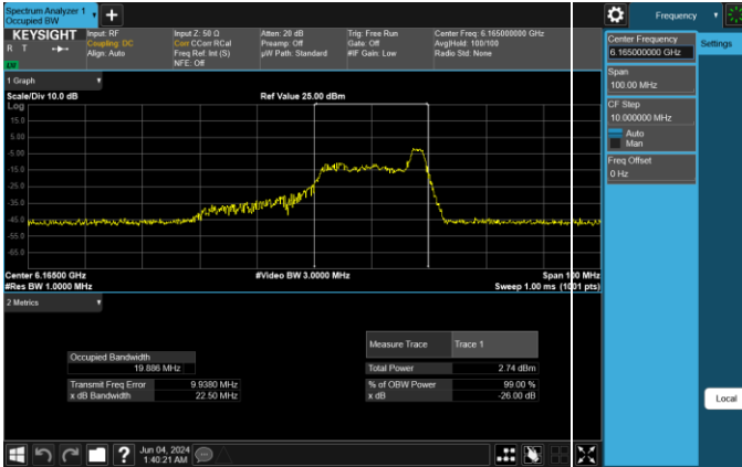
Plot 7-103. 26dB & 99% Bandwidth Plot Antenna 5T LPI (40MHz 802.11ax RU26 (UNII Band 5) – Ch. 43)
