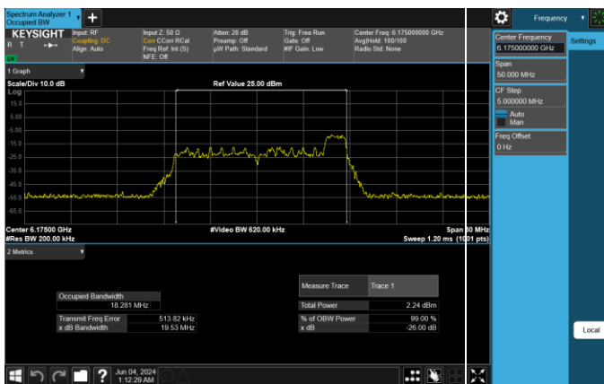
Plot 7-99. 26dB & 99% Bandwidth Plot Antenna 5T LPI (20MHz 802.11ax RU26 (UNII Band 5) – Ch. 45)
