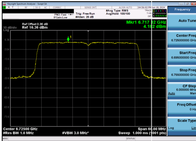
Plot 7-188. Power Spectral Density Plot Antenna 3b SP (40MHz 802.11ax (UNII Band 7) – Ch. 155, MCS11)
