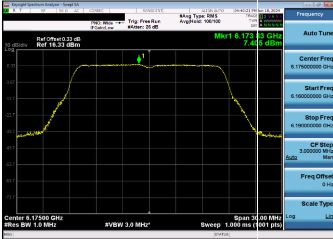
Plot 7-181. Power Spectral Density Plot Antenna 3b SP (20MHz 802.11a (UNII Band 5) – Ch. 45, 54Mbps)
