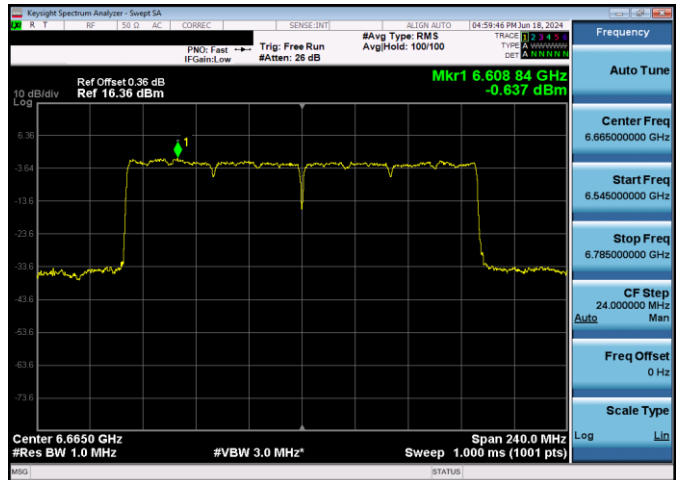
Plot 7-190. Power Spectral Density Plot Antenna 3b SP (160MHz 802.11ax (UNII Band 7) – Ch. 143, MCS11)
