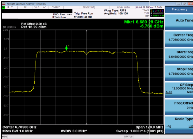
Plot 7-214. Power Spectral Density Plot Antenna 1b LPI (80MHz 802.11ax (UNII Band 7) – Ch. 151, MCS11)
