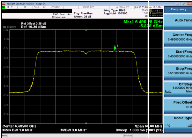
Plot 7-208. Power Spectral Density Plot Antenna 1b LPI (40MHz 802.11ax (UNII Band 6) – Ch. 107, MCS11)
