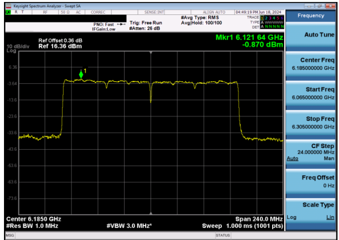
Plot 7-185. Power Spectral Density Plot Antenna 3b SP (160MHz 802.11ax (UNII Band 5) – Ch. 47, MCS11)
