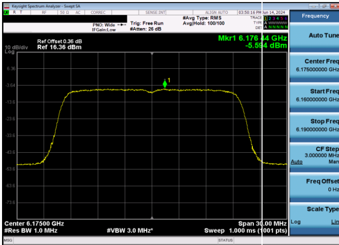
Plot 7-122. Power Spectral Density Plot Antenna 5T LPI (20MHz 802.11ax (UNII Band 5) – Ch. 45, MCS11)
