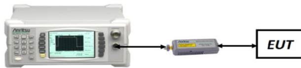
Figure 7-2. Test Instrument & Measurement Setup
