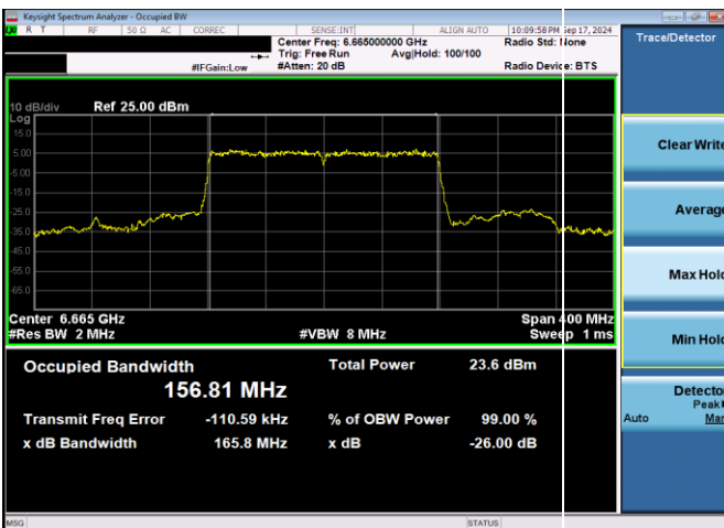
Plot 7-105. 26dB & 99% Bandwidth Plot Antenna 1b LPI (160MHz 802.11ax (UNII Band 7) – Ch. 143, MCS11)
