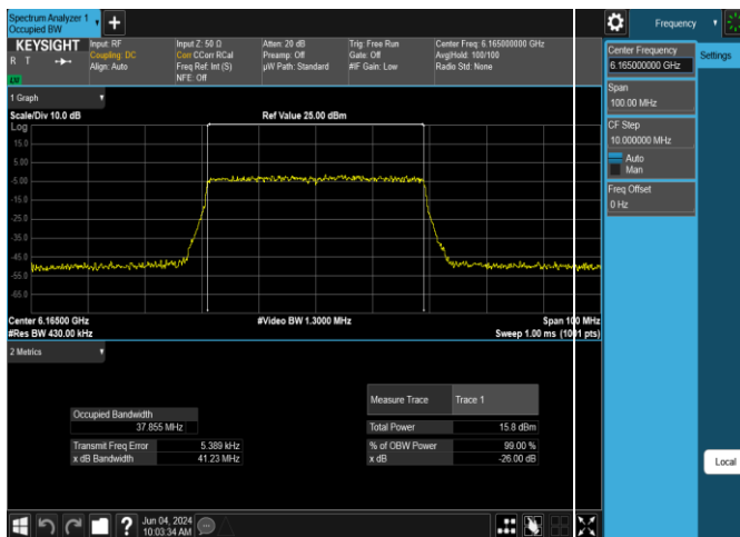
Plot 7-13. 26dB & 99% Bandwidth Plot Antenna 5T LPI (40MHz 802.11ax (UNII Band 5) – Ch. 43, MCS11)
