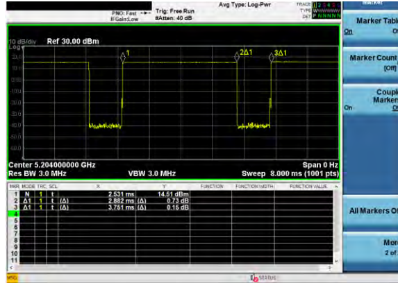
Figure 8-15 NB UNII 1 BDR Transmission Plot – Antenna 5T, Variant 1
