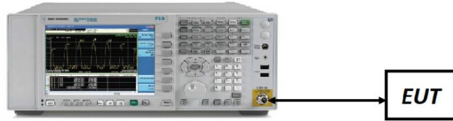
Figure 7-1. Test Instrument & Measurement Setup
