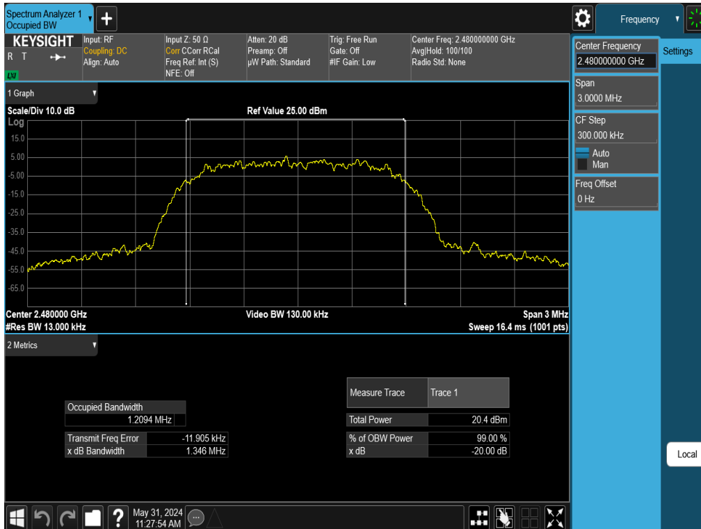
Plot 7-12. 20dB BW and 99% OBW Plot Antenna 1a (Bluetooth, 8DPSK, ePA – Ch. 78)
