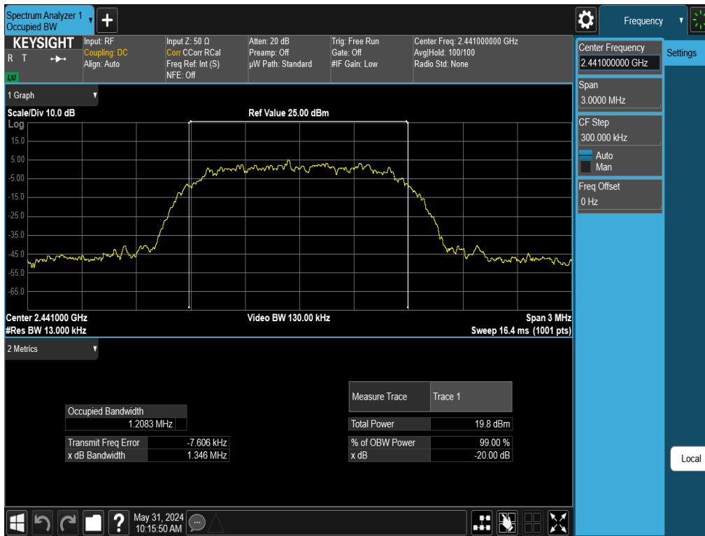
Plot 7-5. 20dB BW and 99% OBW Plot Antenna 3a (Bluetooth, 8DPSK, ePA – Ch. 39)
