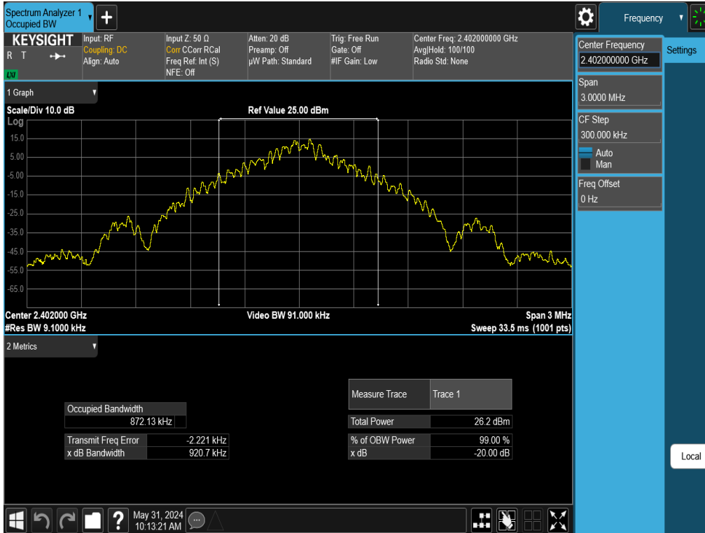
Plot 7-1. 20dB BW and 99% OBW Plot Antenna 3a (Bluetooth, GFSK, ePA – Ch. 0)
