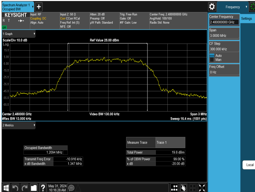
Plot 7-6. 20dB BW and 99% OBW Plot Antenna 3a (Bluetooth, 8DPSK, ePA – Ch. 78)
