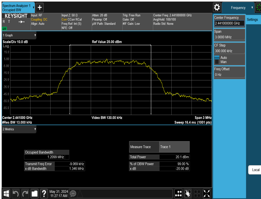
Plot 7-11. 20dB BW and 99% OBW Plot Antenna 1a (Bluetooth, 8DPSK, ePA – Ch. 39)
