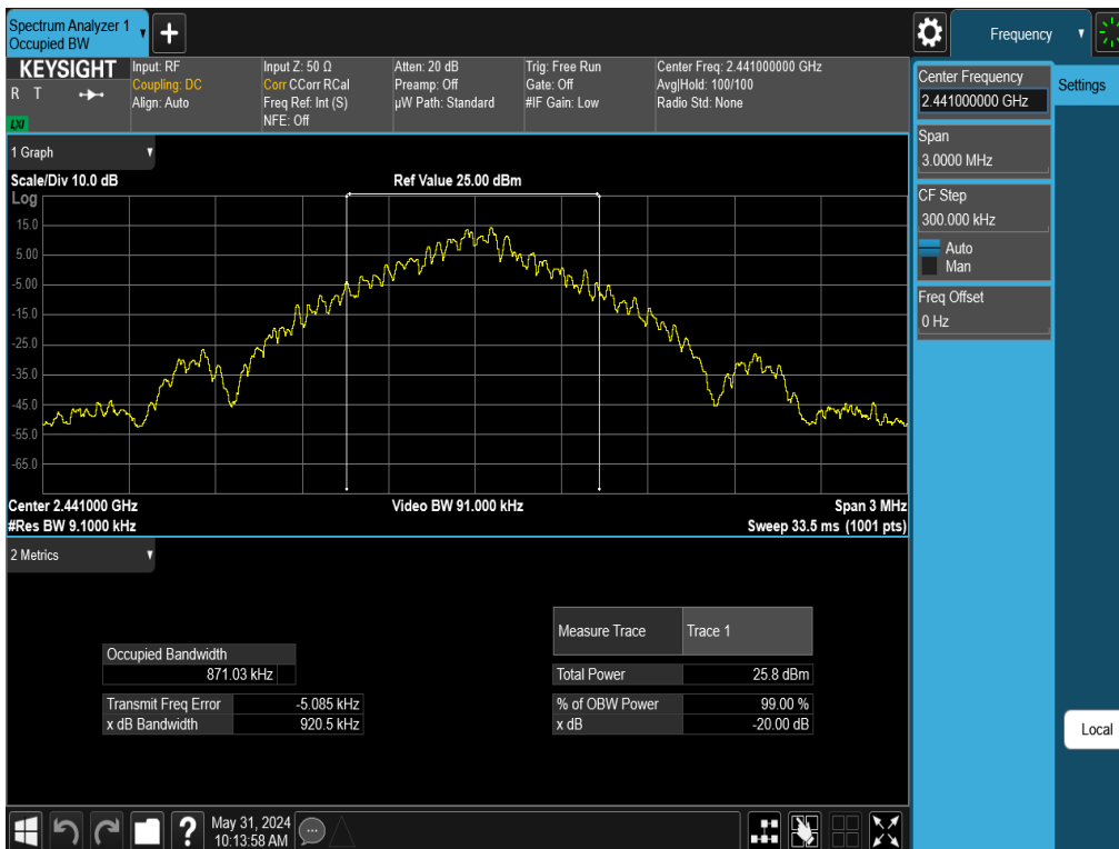
Plot 7-2. 20dB BW and 99% OBW Plot Antenna 3a (Bluetooth, GFSK, ePA – Ch. 39)
