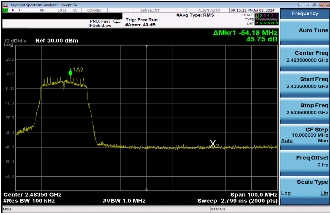
Plot 7-325. Band Edge Plot Antenna 1a (802.11n (2.4GHz) - Ch. 9) - MCS2
