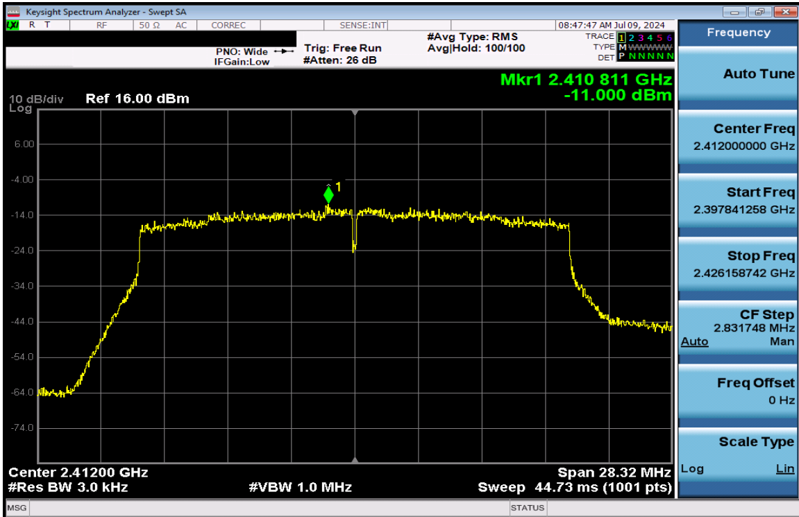
Plot 7-134. Power Spectral Density Plot CDD Antenna 1a (802.11ax (SU - 2.4GHz) – Ch. 1) – MCS2
