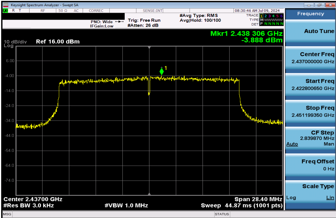
Plot 7-98. Power Spectral Density Plot Antenna 1a (802.11ax (SU - 2.4GHz) – Ch. 6) – MCS2
