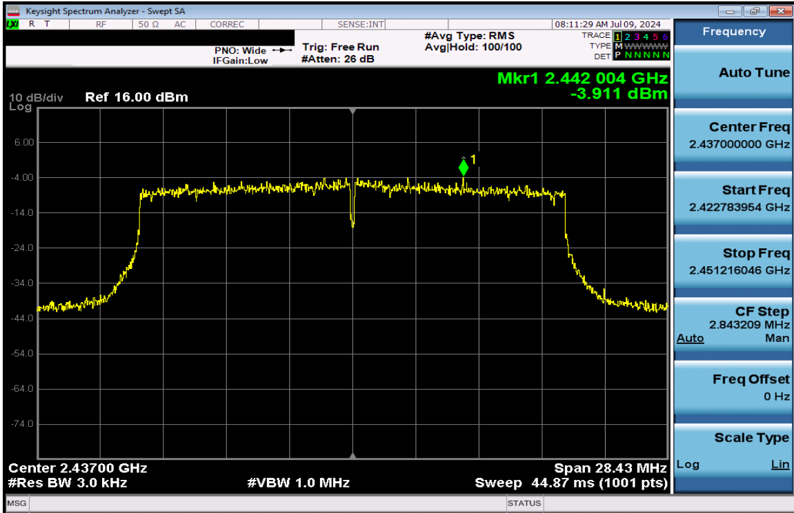
Plot 7-153. Power Spectral Density Plot CDD Antenna 3a (802.11ax (SU - 2.4GHz) – Ch. 6) – MCS4
