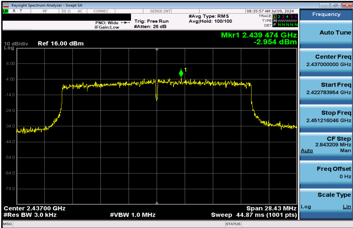
Plot 7-107. Power Spectral Density Plot Antenna 1a (802.11ax (SU - 2.4GHz) – Ch. 6) – MCS4
