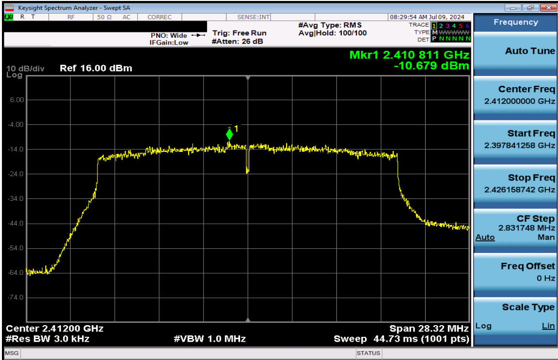
Plot 7-97. Power Spectral Density Plot Antenna 1a (802.11ax (SU - 2.4GHz) – Ch. 1) – MCS2
