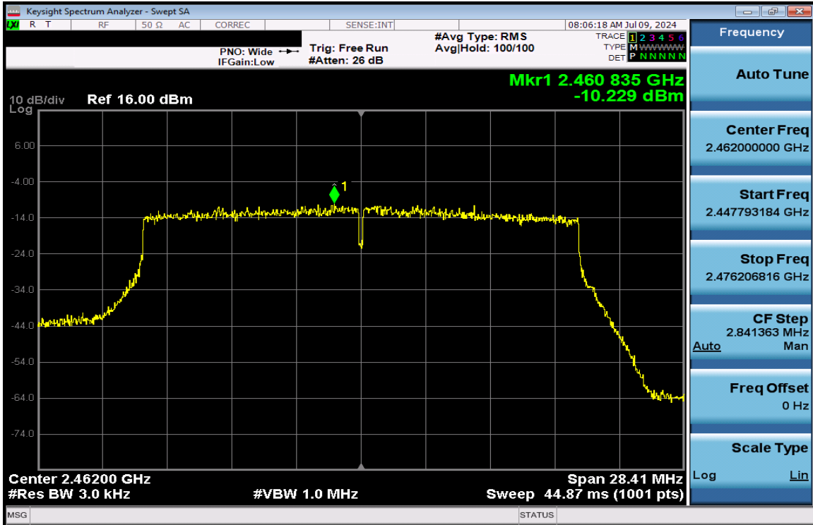
Plot 7-137. Power Spectral Density Plot CDD Antenna 3a (802.11ax (SU - 2.4GHz) – Ch. 11) – MCS2
