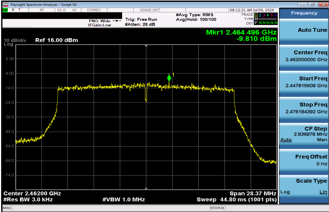
Plot 7-155. Power Spectral Density Plot CDD Antenna 3a (802.11ax (SU - 2.4GHz) – Ch. 11) – MCS4
