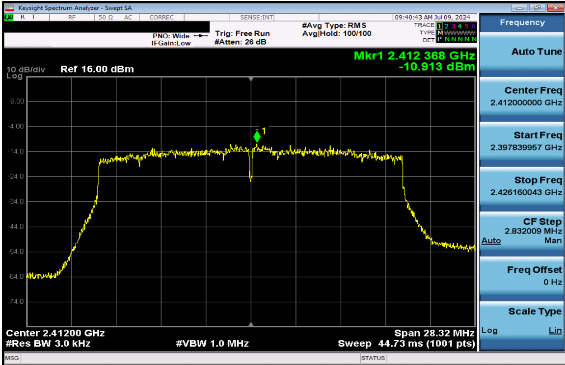
Plot 7-106. Power Spectral Density Plot Antenna 1a (802.11ax (SU - 2.4GHz) – Ch. 1) – MCS4
