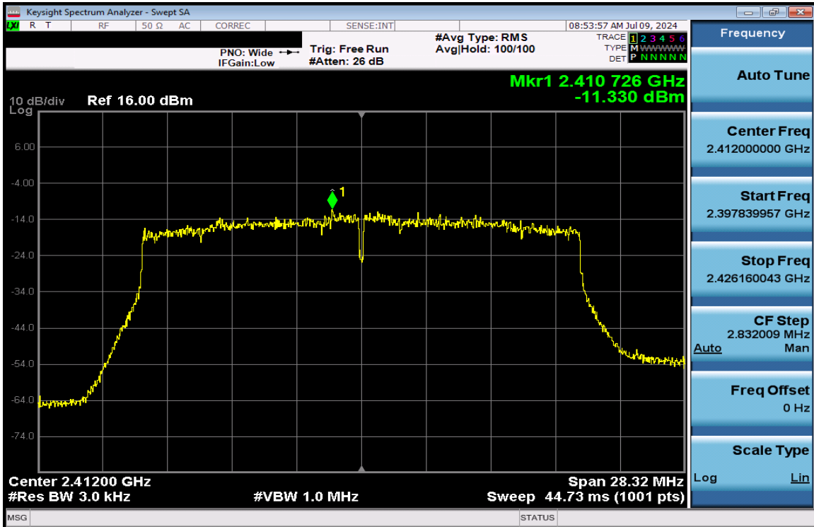
Plot 7-152. Power Spectral Density Plot CDD Antenna 1a (802.11ax (SU - 2.4GHz) – Ch. 1) – MCS4
