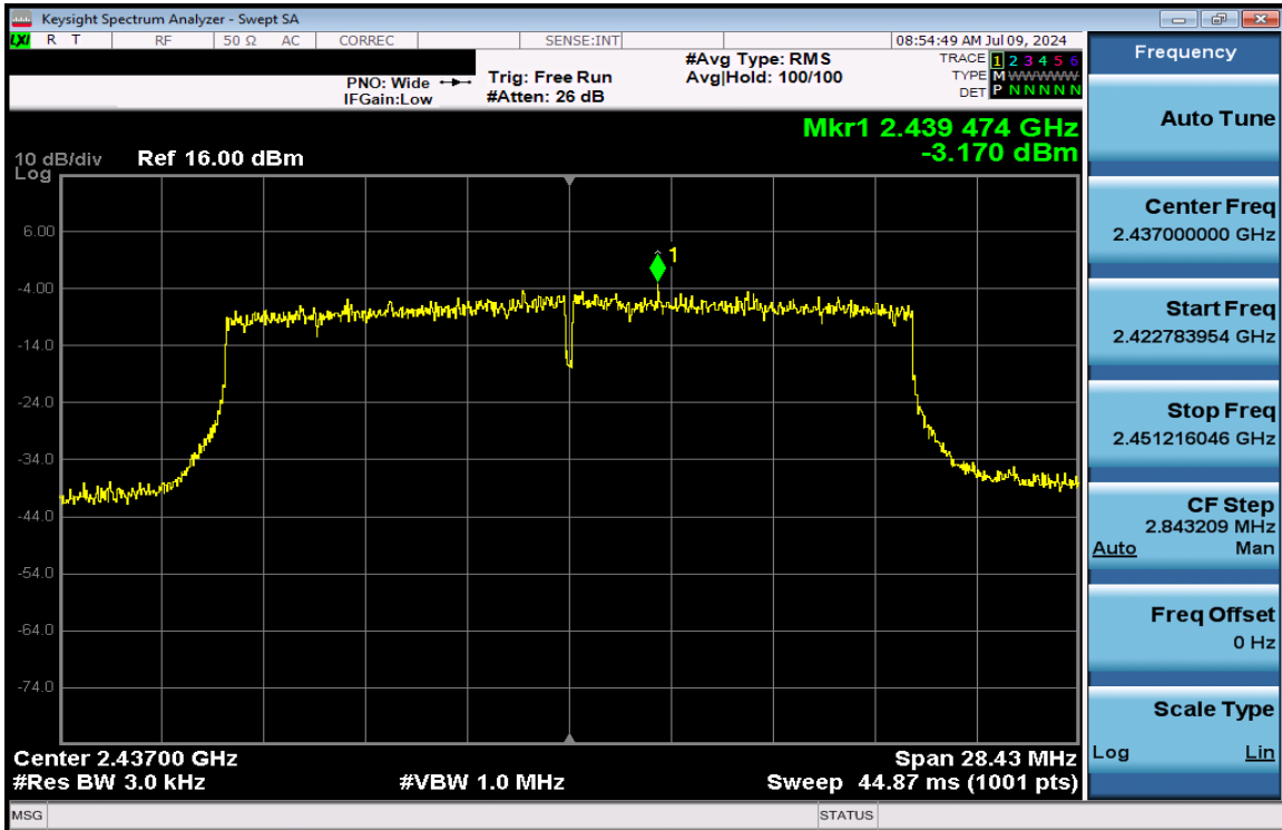
Plot 7-154. Power Spectral Density Plot CDD Antenna 1a (802.11ax (SU - 2.4GHz) – Ch. 6) – MCS4
