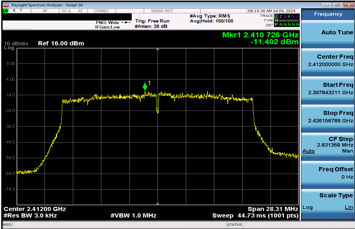
Plot 7-151. Power Spectral Density Plot CDD Antenna 3a (802.11ax (SU - 2.4GHz) – Ch. 1) – MCS4
