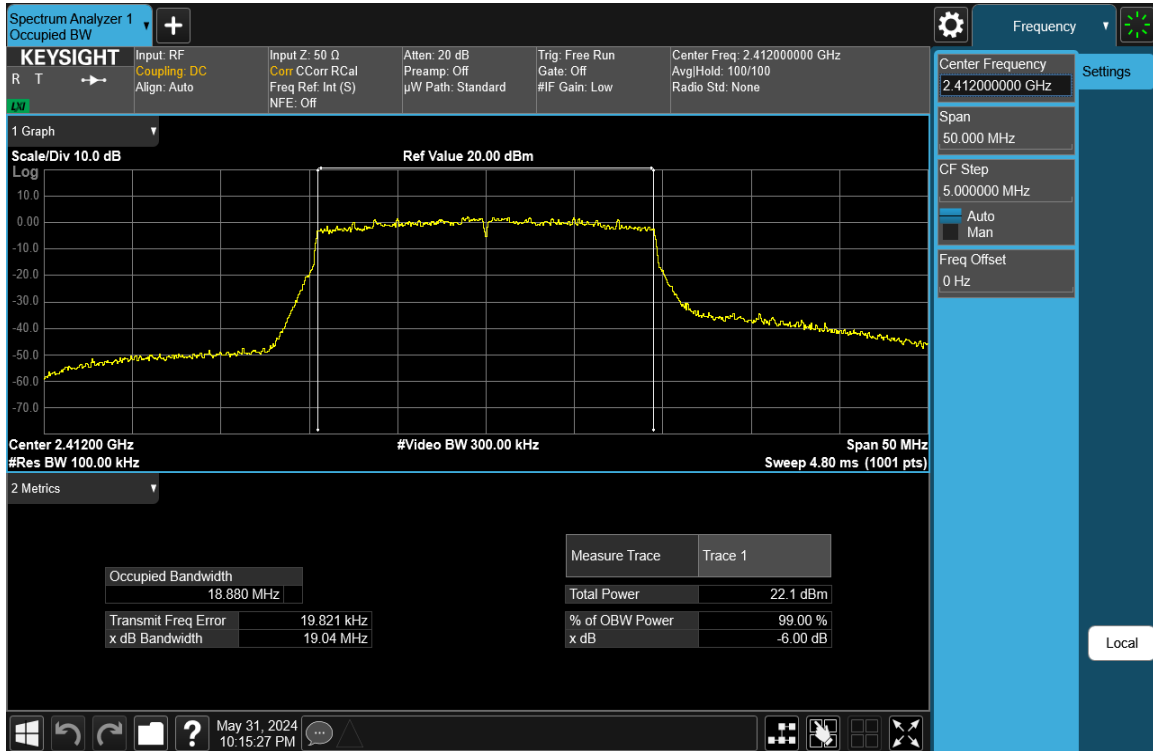
Plot 7-46. 6 dB BW and 99% OBW Plot Antenna 1a (802.11ax (SU - 2.4GHz) – Ch. 1) – MCS4
