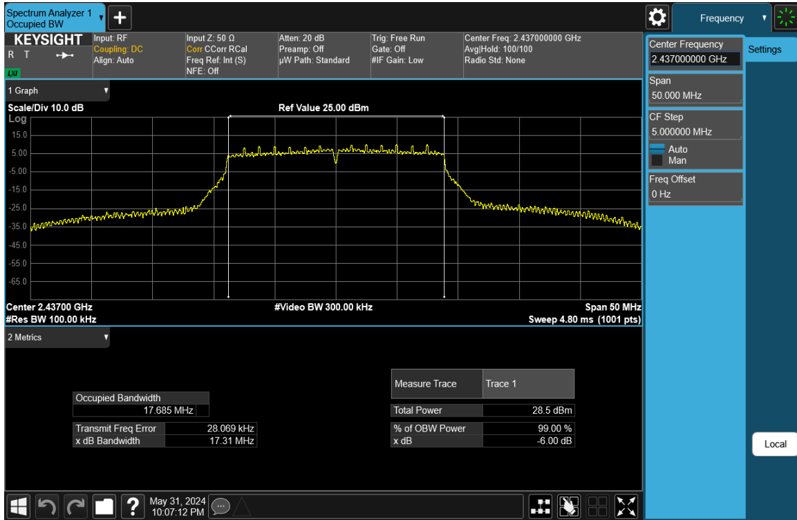
Plot 7-35. 6 dB BW and 99% OBW Plot Antenna 1a (802.11n (2.4GHz) – Ch. 6) – MCS2
