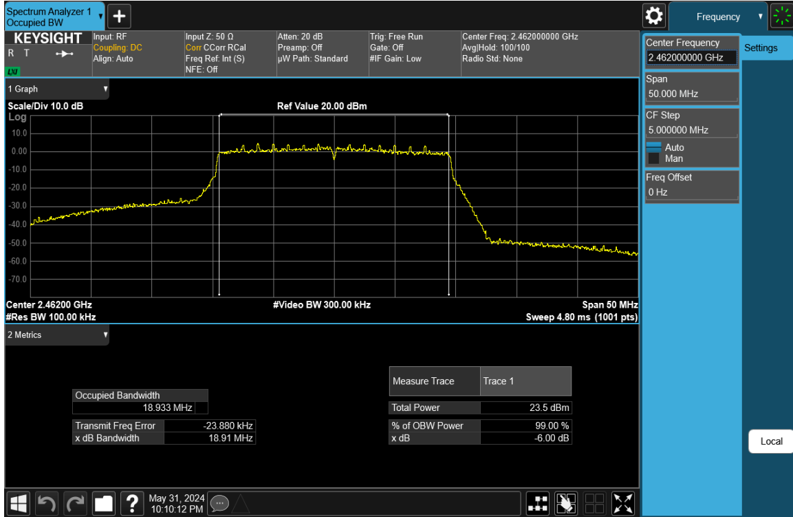
Plot 7-39. 6 dB BW and 99% OBW Plot Antenna 1a (802.11ax (SU - 2.4GHz) – Ch. 11) – MCS2
