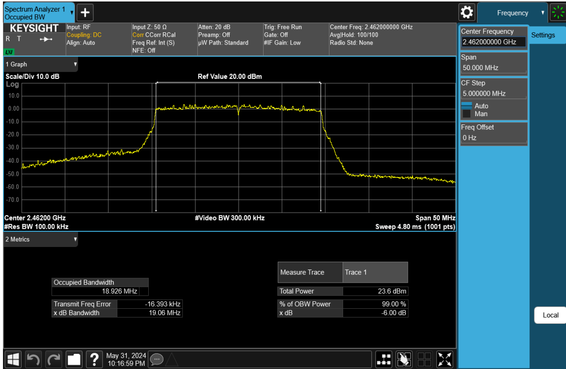
Plot 7-48. 6 dB BW and 99% OBW Plot Antenna 1a (802.11ax (SU - 2.4GHz) – Ch. 11) – MCS4
