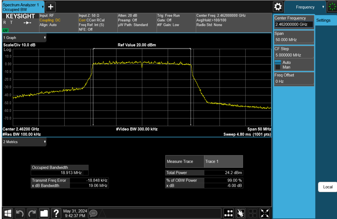
Plot 7-18. 6 dB BW and 99% OBW Plot Antenna 3a (802.11ax (SU - 2.4GHz) – Ch. 11) – MCS4
