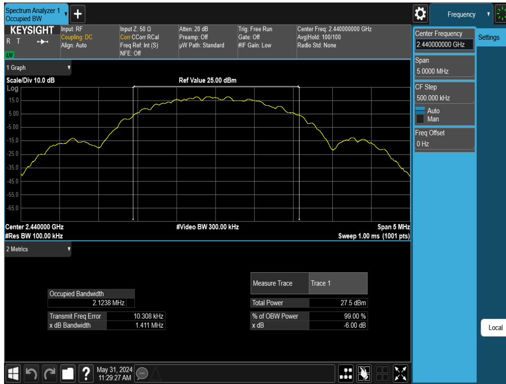
Plot 7-11. 6dB BW & 99% OBW Plot Antenna 1a (Bluetooth (LE), 2Mbps, ePA – Ch. 19)
