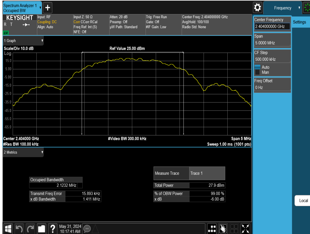
Plot 7-4. 6dB BW & 99% OBW Plot Antenna 3a (Bluetooth (LE), 2Mbps, ePA – Ch. 1)
