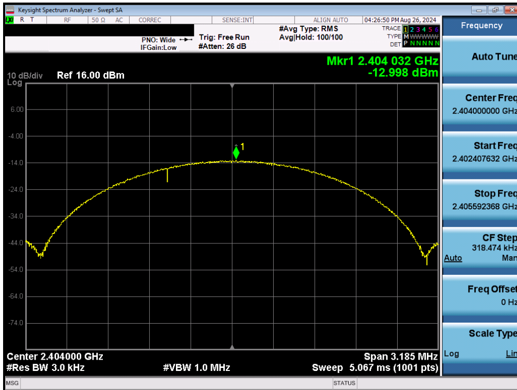
Plot 7-67. Power Spectral Density Plot Antenna 3a (Bluetooth (LE), 2Mbps, iPA – Ch. 1)
