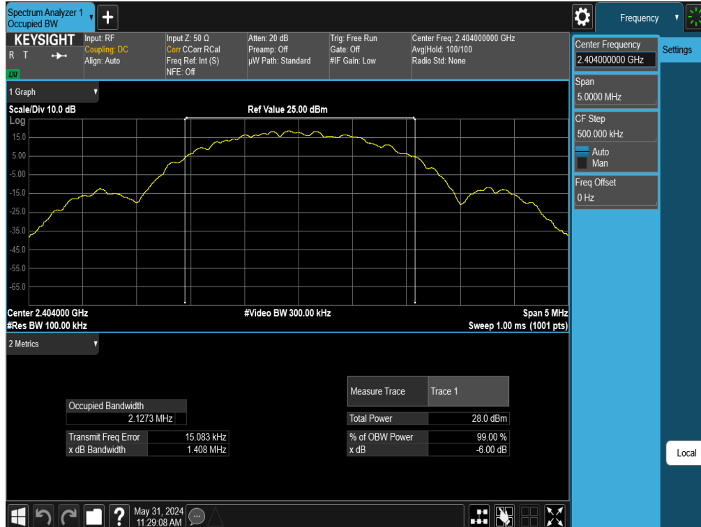
Plot 7-10. 6dB BW & 99% OBW Plot Antenna 1a (Bluetooth (LE), 2Mbps, ePA – Ch. 1)
