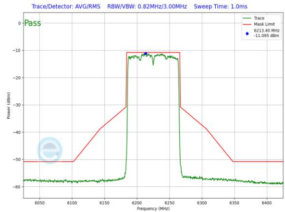
Plot 7-298. In-Band Emission Plot Antenna WF2 VLP (80MHz 802.11ax (UNII Band 5) – Ch. 55, MCS11)
