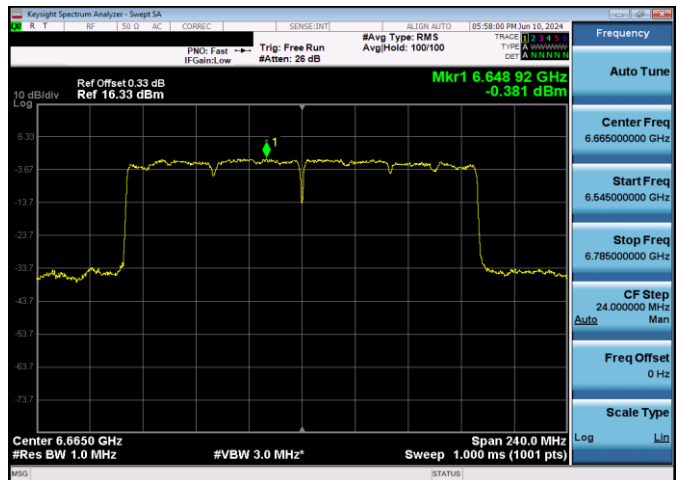
Plot 7-208. Power Spectral Density Plot CDD Antenna WF2 SP (160MHz 802.11ax (UNII Band 7) – Ch. 143, MCS11)
