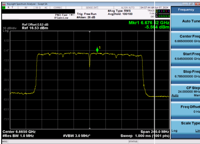
Plot 7-95. Power Spectral Density Plot Antenna WF5T LPI (160MHz 802.11ax (UNII Band 7) – Ch. 143, MCS11)
