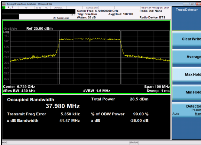
Plot 7-48. 26dB & 99% Bandwidth Plot Antenna WF2 SP (40MHz 802.11ax (UNII Band 7) – Ch. 155, MCS11)
