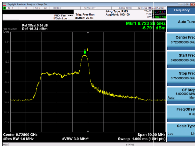
Plot 7-482. LPI Power Spectral Density Plot Antenna WF2 (40MHz 802.11ax RU26 (UNII Band 7) – Ch. 155)
