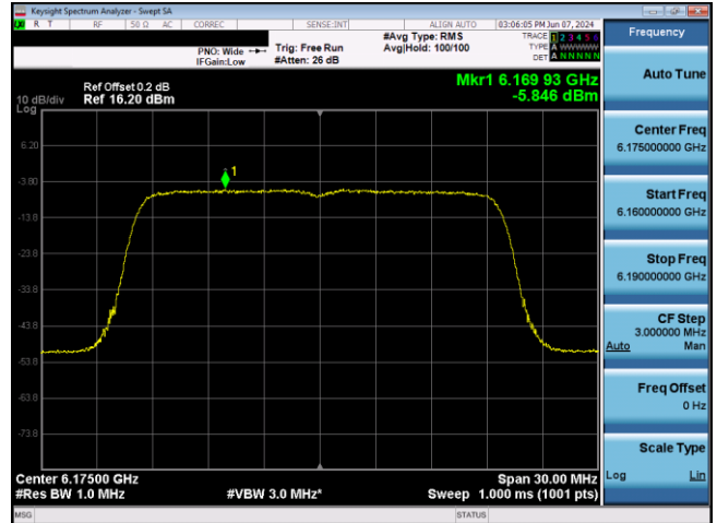
Plot 7-448. LPI Power Spectral Density Plot Antenna WF2 (20MHz 802.11ax RU242 (UNII Band 5) – Ch. 45)
