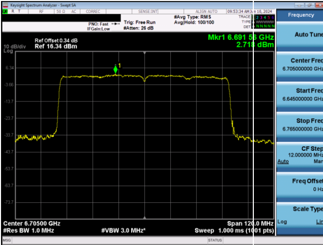
Plot 7-371. SP Power Spectral Density Plot SDM Antenna WF5T (80MHz 802.11ax RU996 (UNII Band 7) – Ch. 151)
