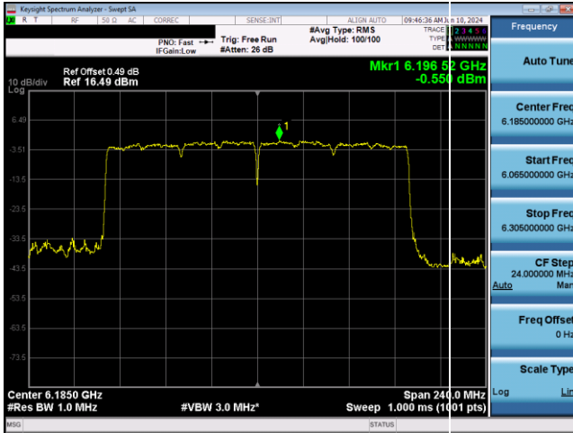
Plot 7-347. SP Power Spectral Density Plot SDM Antenna WF5T (160MHz) 802.11ax RU996x2 (UNII Band 5) – Ch. 47)
