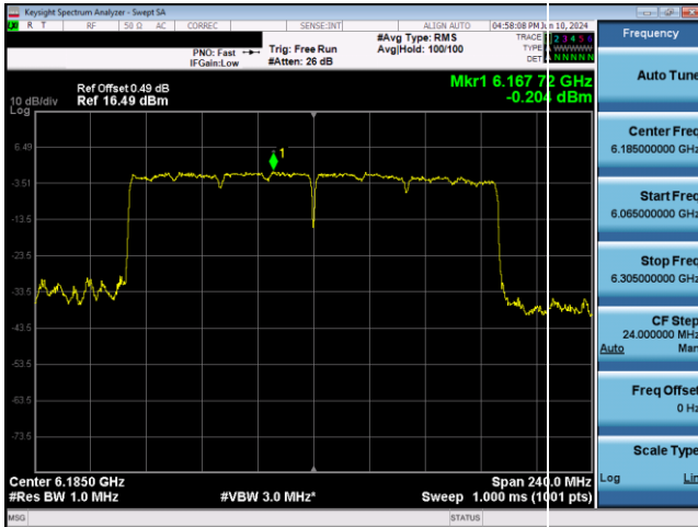
Plot 7-348. SP Power Spectral Density Plot SDM Antenna WF2 (160MHz) 802.11ax RU996x2 (UNII Band 5) – Ch. 47)
