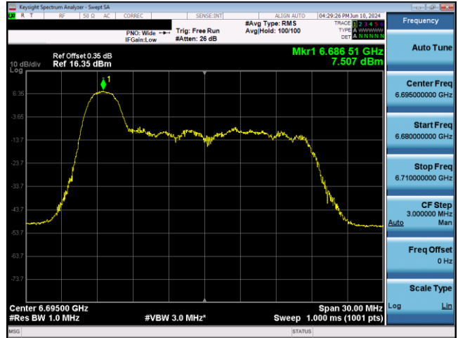
Plot 7-350. SP Power Spectral Density Plot SDM Antenna WF2 (20MHz) 802.11ax RU26 (UNII Band 7) – Ch. 149)
